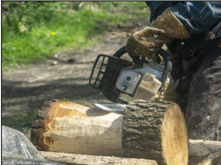
Using the edge of the blade to smooth the "stalk".
