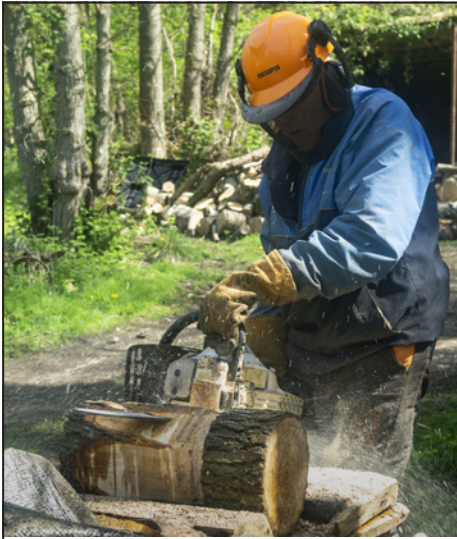
Shaving the "stalk" is an iterative process, taking a sliver off each rotation.
