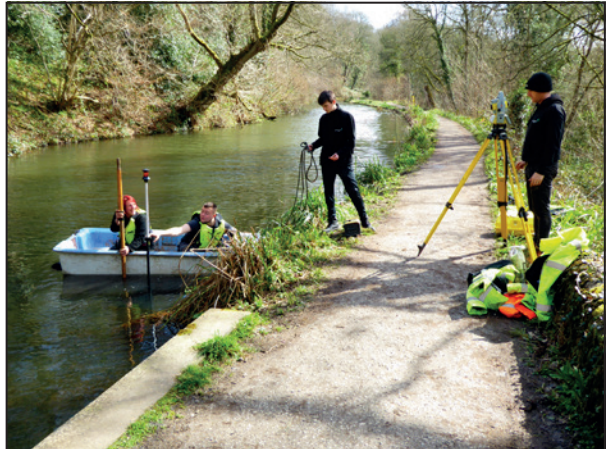
Techniques old and new were used to measure the profile of the canal bed between Aqueduct Cottage and Gregory Tunnel.
