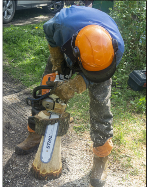
Cutting the taper on the "cap" is also an iterative process, like the "stalk". It is made more difficult because the mushroom is not supported.
